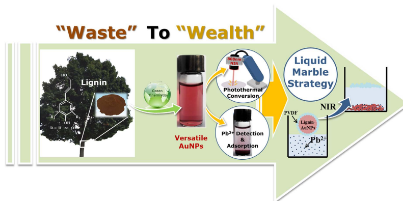
Figure 1. Illustration of this study: lignin is used to synthesize versatile AuNPs, and a novel liquid marble strategy was employed to combine the photothermal conversion and simultaneous Pb 2+ detection and adsorption properties of the lignin-AuNPs composites, resulting in NIR-responsive lignin-AuNPs liquid marbles.
